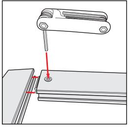
Extrusion & Lock Connection
