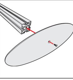
Base Plate & Extrusion Connection
